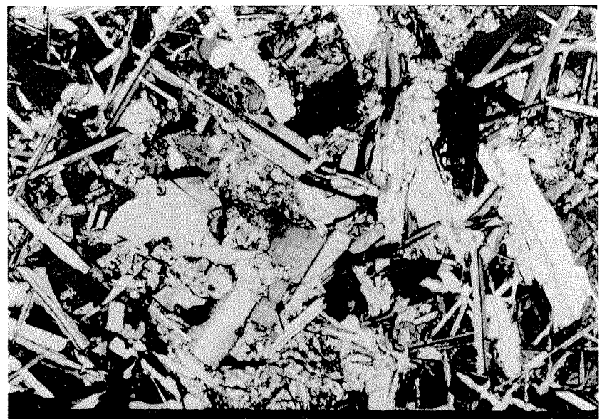
FIGURE 2.8.—Crystalline, igneous-appearing texture of impact-melt rock (James, 1973), sample 14310,170 from Apollo 14 landing site. Texture is partly subophitic, like that of basalt sample in figure 2.6A, and partly intersertal (fine-grained minerals in interstices of larger plagioclase crystals).
