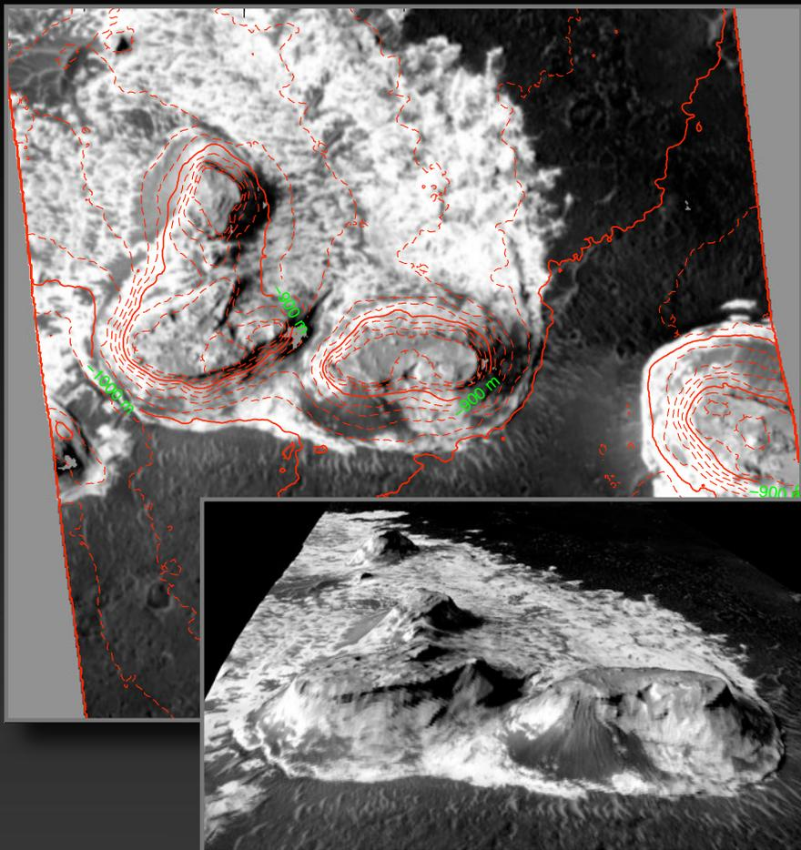
Above Left: This DEM was generated from MOC images E04-01109 and M20-01357 (2.38°N, 6.40°E). The contour lines (20m spacing) overlay an ortho-image generated from the 3D terrain model.
