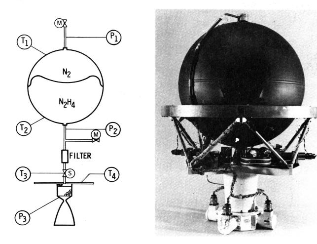
The Mariner 10 spacecraft uses a self-contained monopropellant hydrazine propulsion subsystem to provide the velocity changes necessary to remove launch vehicle errors and for the in-transit trajectory correction maneuvers (TCM) required to achieve the desired flybys of the planets Venus and Mercury.
